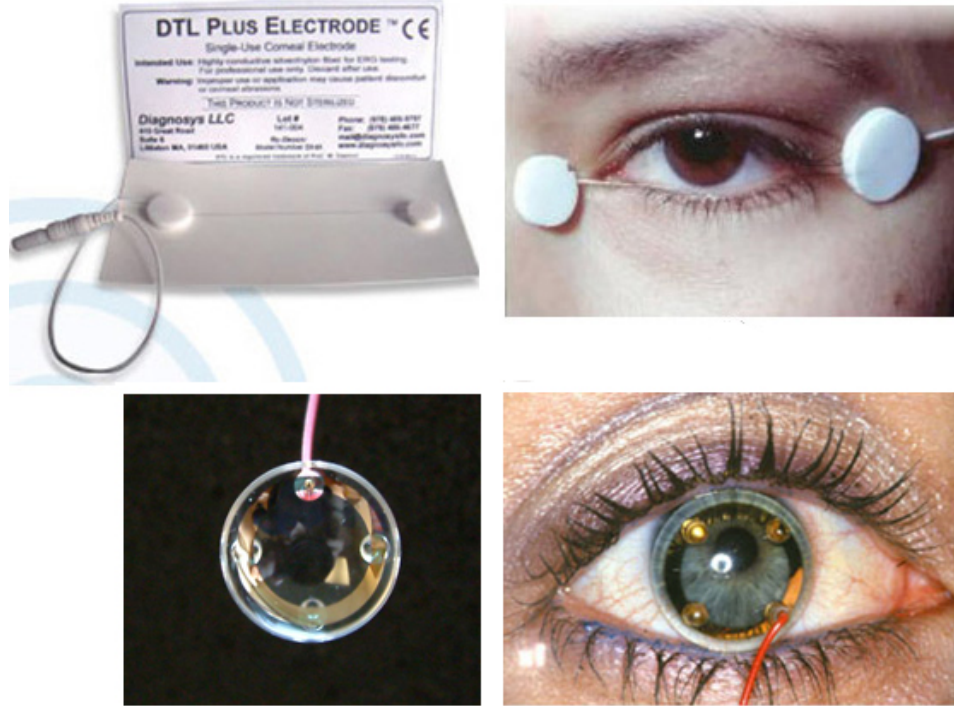
Figure 4.3: DTL Plus electrode, courtesy of Diagnosys LLC ( www.diagnosysllc.com ), by its own (Top Left), and positioned on eye (Top Right). ERG-Jet corneal electrode, courtesy of Fabrinal SA ( www.fabrinal.ch ), by its own (Bottom Left) and placed on eye (Bottom Right).
